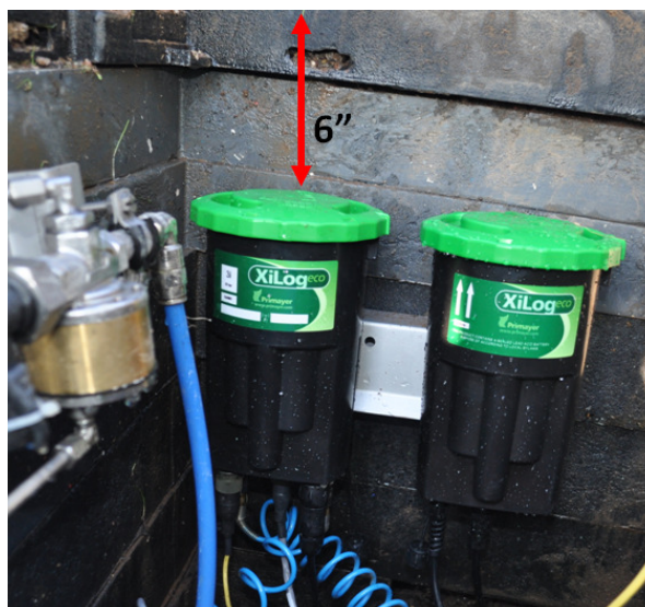
Picture shows XiLogEco in recommended position inside a chamber.
